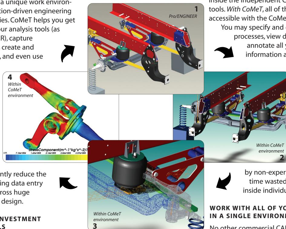
1-2: Import a Pro/ENGINEER assembly into CoMeT, and automatically create joints, springs, bushings, dampers, etc. for analysis using MSC.Adams for rigid and flex body analysis.
